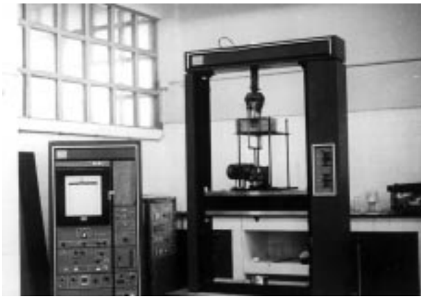
Figure 2 Overall view of the installations showing the Instron tensile strength tester.
